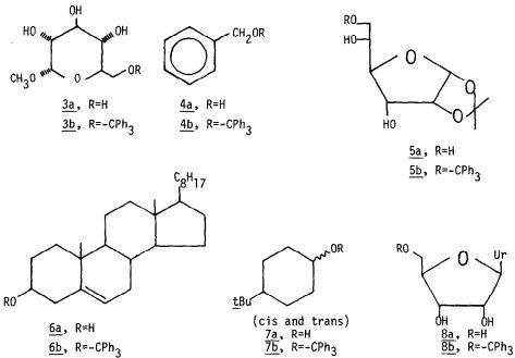
This combination of reagents is also effective in solvents other than DMF as shown by formation of  $\underline{4b}$  (90%) in dichloromethane solution at room temperature. Reaction of secondary alcohols is considerably slower (18-24 hr) and requires higher temperatures (40-45°), thus the trityl ethers  $\underline{6b}$  and  $\underline{7b}$  were prepared in refluxing dichloromethane (68% and 70%) and in DMF solution at 45° ( $\underline{7b}$ ,  $\underline{65\%}$ ).
